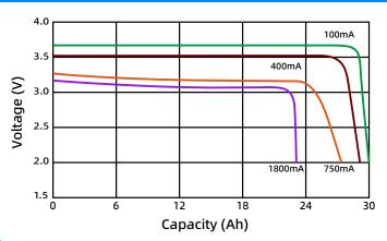
2. Voltage graphs at different discharge currents and temperatures (during the stabilisation phase of the discharge)
