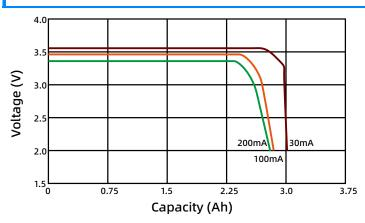
2. Voltage graphs at different discharge currents and temperatures (during the stabilisation phase of the discharge)
